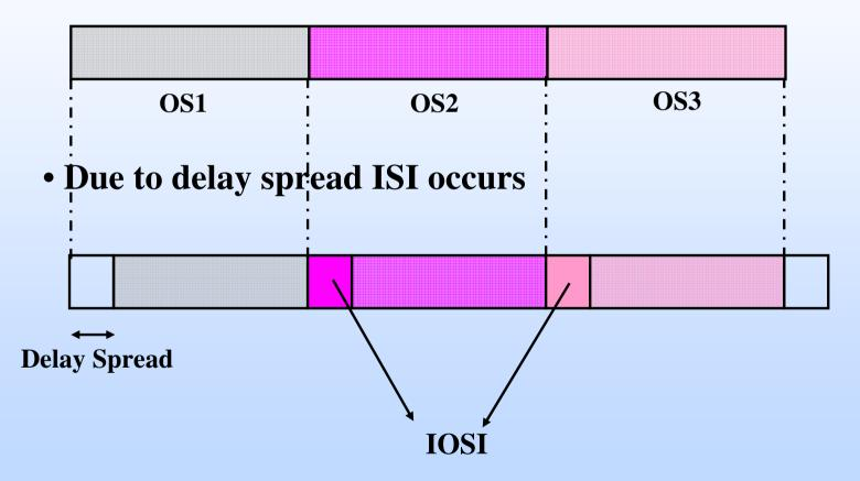
• Solution could be guard interval between OFDM symbols
