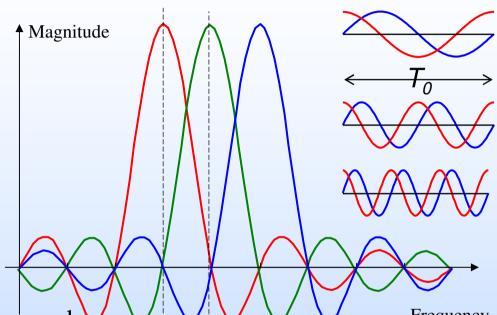
Subcarrier orthogonality must be preserved  $\checkmark \lor \lor \lor \lor \lor \lor$ Compromised by timing jitter, frequency offset, and fading. Frequency
