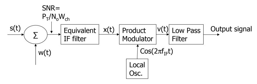
• Consider DSB-TC  $s(t) = A_c[1 + k_a m(t)]\cos(2\pi f_c t)$  where m(t) is considered a sample function of a stationary process of zero mean and PSD  $S_M(f)$  limited to maximum frequency W as shown in the next slide
