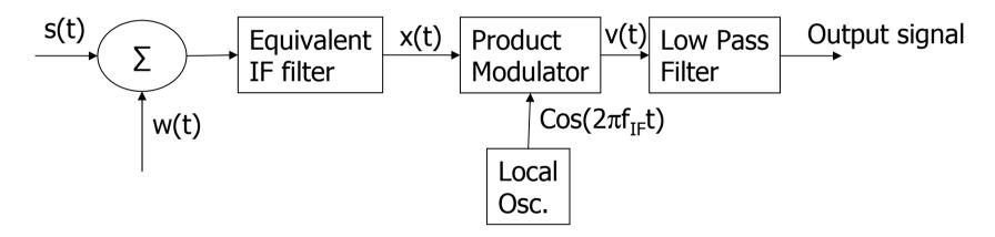
• Consider DSB-SC  $s(t) = A_c \cos(2\pi f_c t) m(t)$  where m(t) is considered a sample function of a stationary process of zero mean and PSD  $S_M(f)$  limited to maximum frequency W as shown in the next slide
