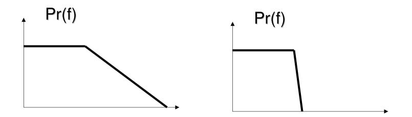
In practical systems where the bandwidth available for transmitting data at a rate of  $r_b$  bits\sec is between  $r_b\2$  to  $r_b$ Hz, a class of  $p_r(t)$  with a *raised cosine frequency characteristic* is most commonly used.
