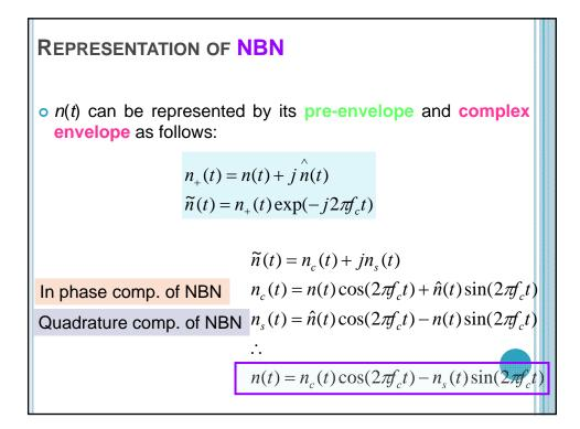
PROPERTIES OF INPHASE AND QUADRATURE COMPONENTS OF NBN 1. If n(t) is zero mean then  $n_c(t)$  and  $n_s(t)$  are also zero mean 2. If n(t) is Gaussian RP then  $n_c(t)$  and  $n_s(t)$  are jointly Gaussian 3. If n(t) is WSS then  $n_c(t)$  and  $n_s(t)$  are jointly WSS  $R_{N_c}(\tau) = R_{N_s}(\tau) = R_N(\tau)\cos(2\pi f_c\tau) + \hat{R}_N(\tau)\sin(2\pi f_c\tau)$ Crosscorrelation  $R_{N_cN_s}(\tau) = -R_{N_sN_c}(\tau) = R_N(\tau)\sin(2\pi f_c\tau) - \hat{R}_N(\tau)\cos(2\pi f_c\tau)$
