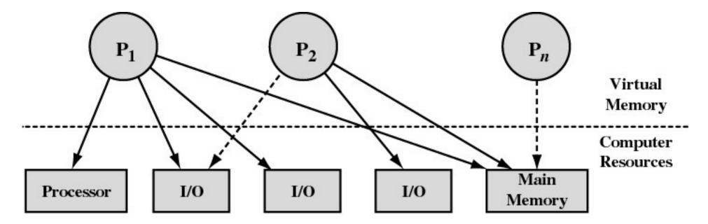
$P_1$ : running, part in main memory, has control of 2 I/O devices
